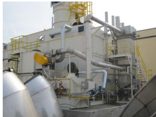
Figure 3. Typical FBC Installation
